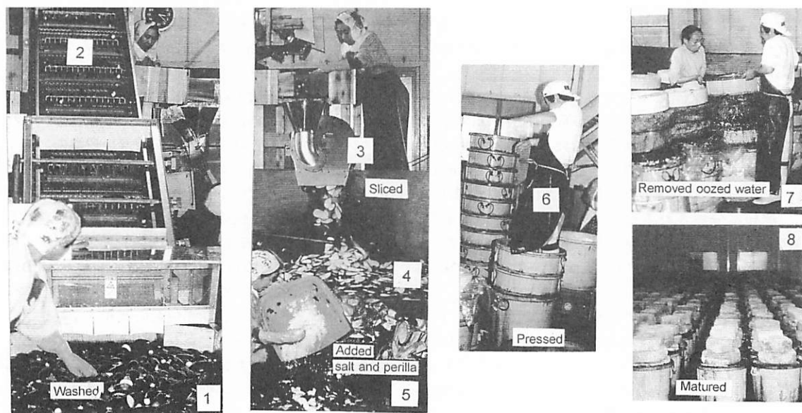
Fig.1 Process of Shibazuke manufacture
